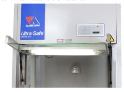
To open the window, pull it firmly outwards. It will support itself in the open position. To close the window, push it down towards the closed position. If the viewing window is opened when the cabinet is running, a boost mode, which activates maximum exhaust airflow and the alarm system, is automatically
